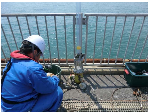
We used vibrator to take core samples.
