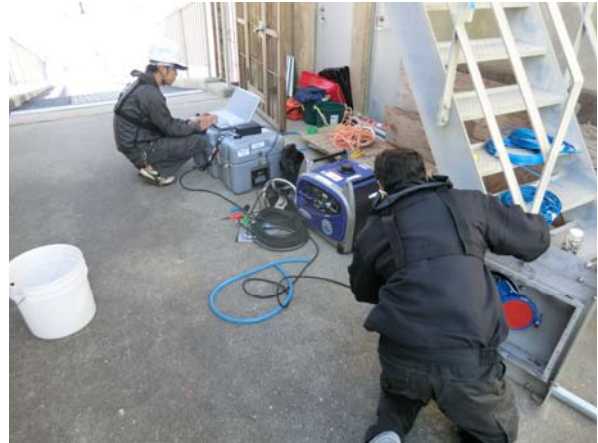
Preparation of H-ADCP
