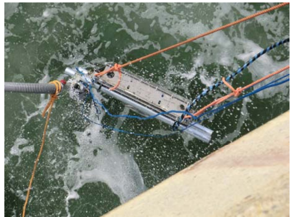
Installation of instrument array, which consist of H-ADCP, wave gage and current meter.
