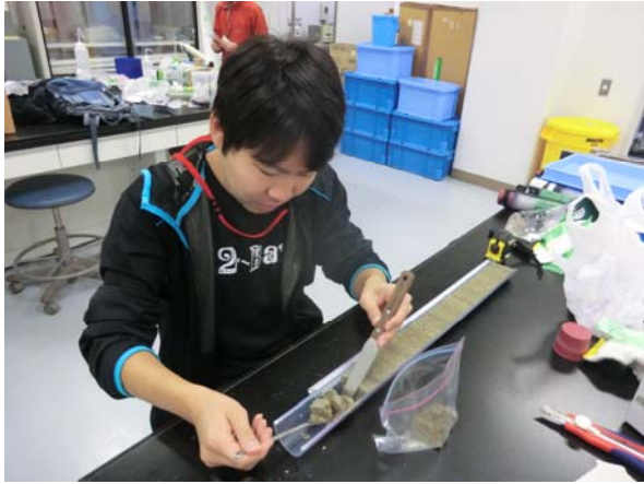
Core sampled sand are sub-divided every 2.5 cm.
